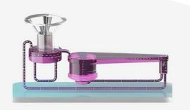
Perfusion around the plate and through the scaffold enables the formation of 3D tissue
